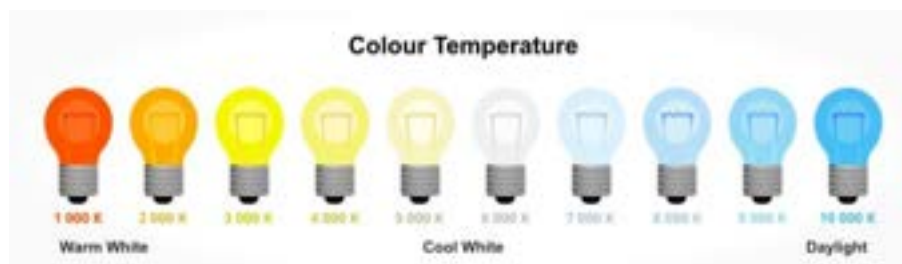
Slika 2: Barvna temperatura Vir: https://www.mjlighting.net/led-lamps
